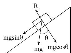
Force by plane on block is equal to reaction
